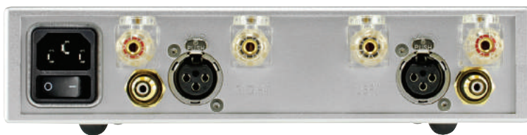
The TToby's power supply is built in, an IEC mains socket and adjacent but inconveniently located mains switch show. Robust quality 'speaker terminals and unbalanced (phono) and balanced (XLR) inputs are fitted. Only one can be connected though.
