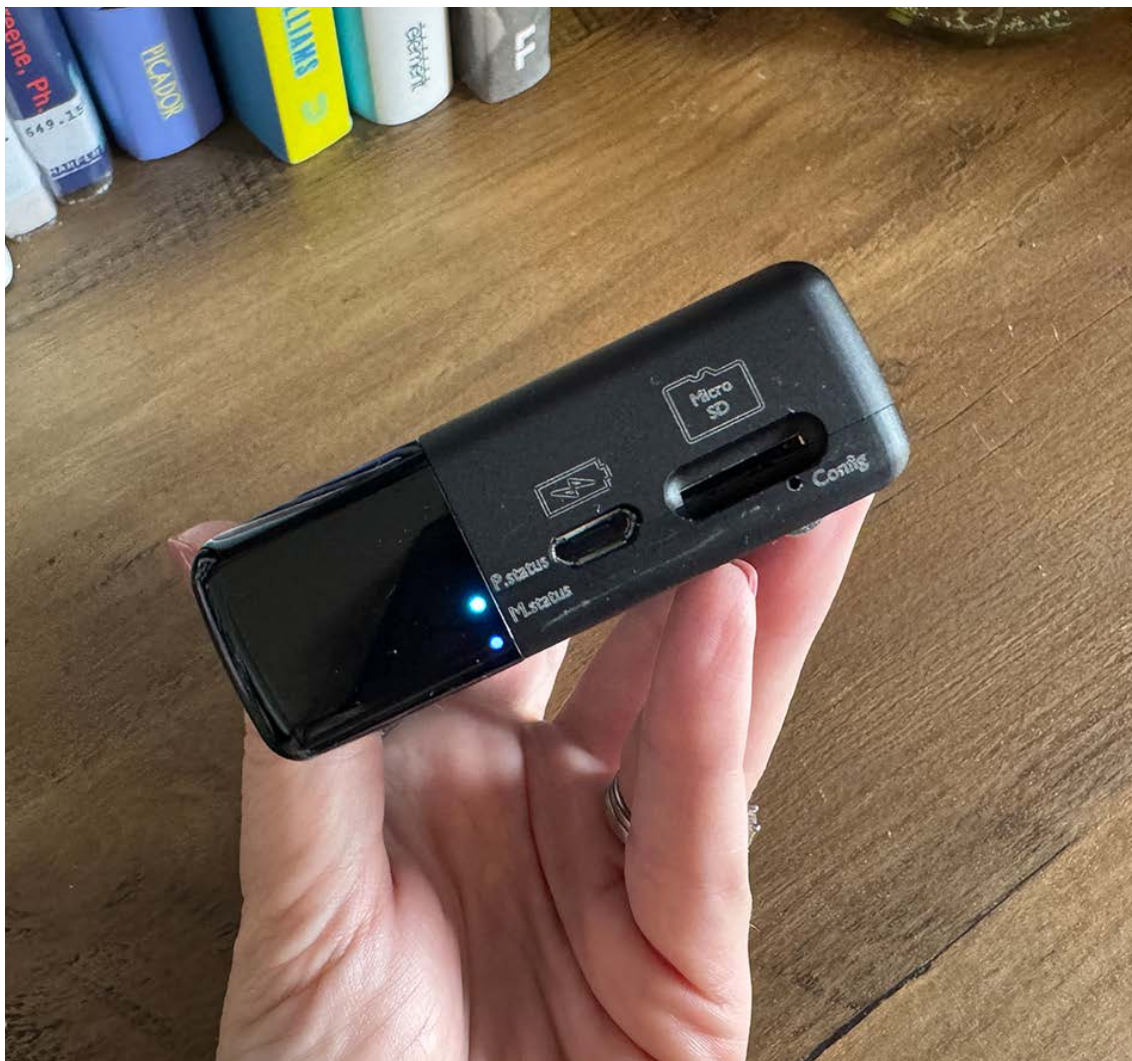
MicroSD card slot allows hi-res music playback from locally stored media
