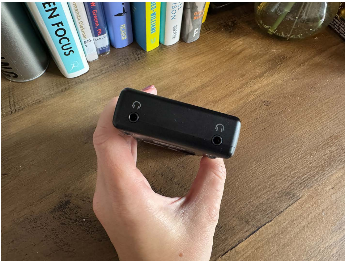
Even better to share – twin 3.5mm headphone outputs for driving a range of cans
